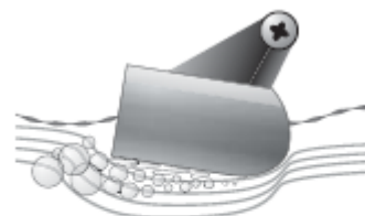
Cavitation that will cause erratic sonar readings
